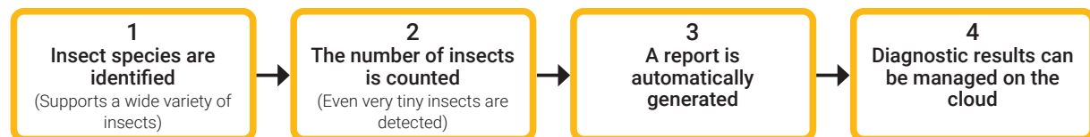
Insects captured on a sticky paper trap are identified and counted using AI.
